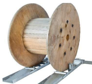
Fig. 2.15: Cable drum blocked using a flange
