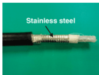
Fig. 1.14: Appearance of high-strength sheath cable
