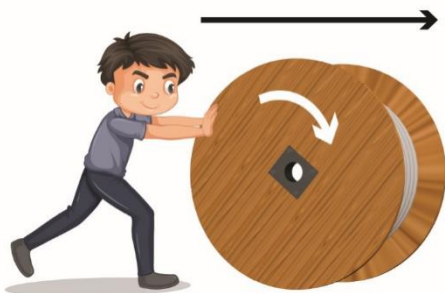
Fig. 2.11: Correct way to roll the cable drum
