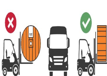
Fig. 2.7: (b) Way to lift and place the cable drum
