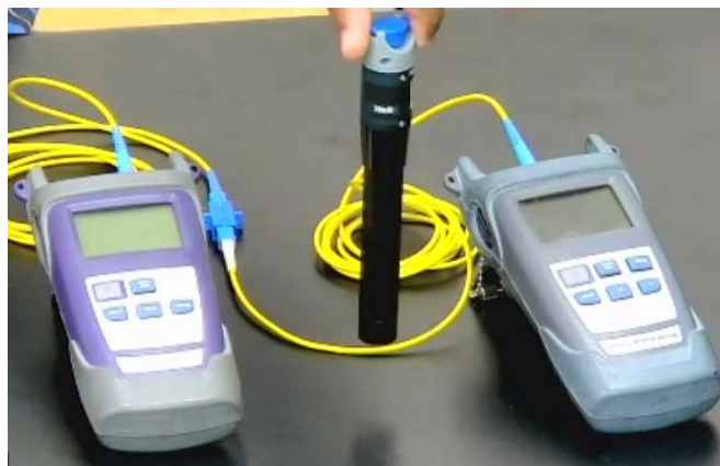
Fig. 1.8: Light source and power meter combination to check the total loss in the fiber
