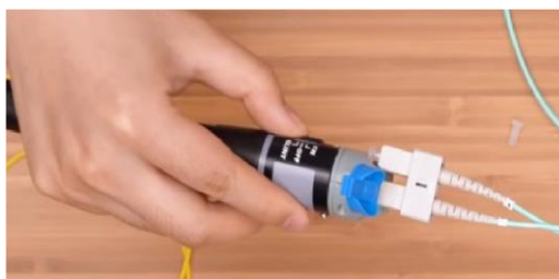
Fig. 3.11: Connecting VFL to SC connector
