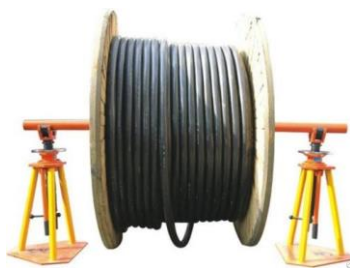
Fig. 4.16: Cable drum stand
