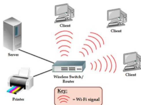
Fig. 2.15 (c) Devices connected to the network using wireless technology.
