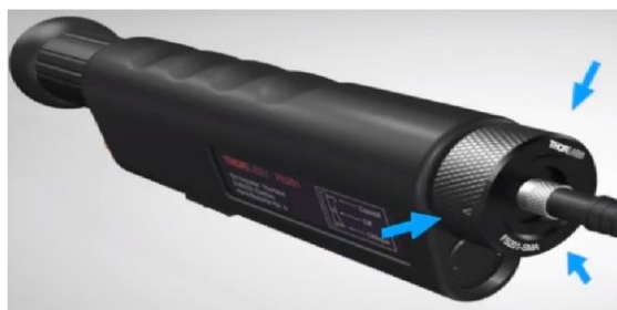
Fig. 3.19: Adjust the screw of the connector adapter
