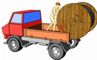
Fig. 2.10: Wrong method of unloading the Drum
