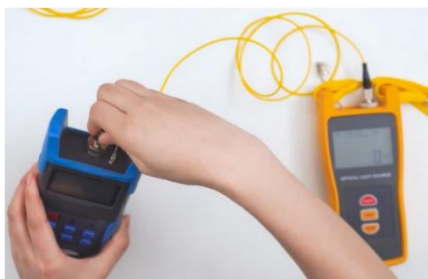
Fig. 3.6 Connecting reference cord to optical power meter and optical light source
