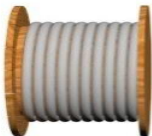
Fig. 2.13: Correct way to place the cable
