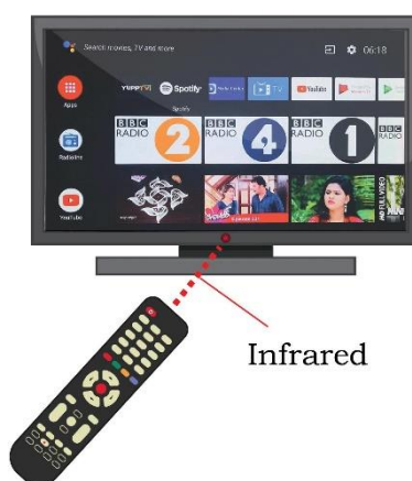
Fig. 2.21: Infrared light wave used in television remote
