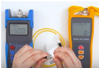
Fig. 3.5 Clean the ends of the reference cord
