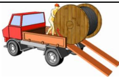
Fig. 2.9: Cable Drum being unloaded from the Ramp carefully
