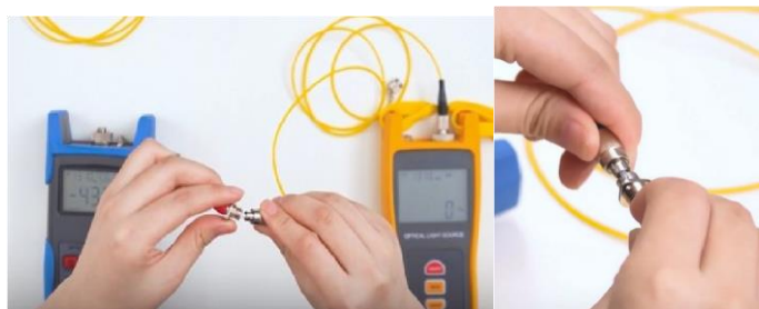
Fig. 3.8 Connect the test cable to the light source
