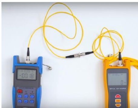
Fig. 3.8 Reading in the optical power meter
