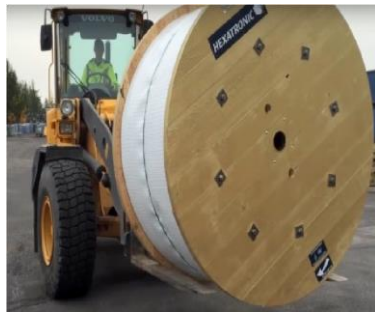
Fig. 2.5: Unloading of cable drum using a forklift.
