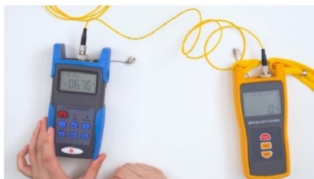
Fig. 3.3 Connecting optical fibre cable to light source
