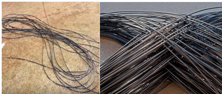
Fig. 4.14: Wrong way to put the optical fibre cable on the floor
